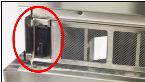
12. Remove the USB and close the front filter cover.
